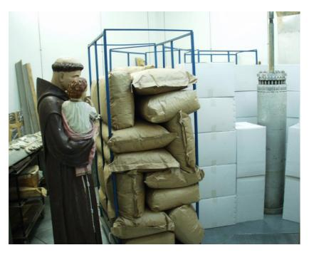
Photo: Simultaneously irradiation of different products in the panoramic gamma facility at the RBI
