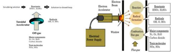
Principle of off gases treatment by electron beam, wet srubber is the second stage
