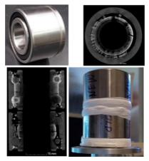
A comparative neutron imaging study of a new and a damaged ball bearing at the RAD station revealed the importance of proper lubrication. (Credits: Zoltán Kis, László Szentmiklósi, László Rosta; Rogante Engineering Office, Italy)
