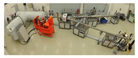
The 3 MV HVE Tandetron<sup>™</sup> accelerator and three high-energy research beamlines (with L1 on the right, L2 in the middle, and L3 on the left) of RoCIBA
