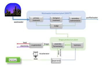
Scheme of biogas and eb plant for safe organic fertilizer manufacturing. A.G.Chmielewski, Electron Accelerators for Environmental Protection, January 2011,Reviews of Accelerator Science and Technology 4:147–159 DOI: 10.1142/9789814383998\_0007
